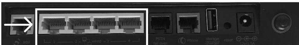
6. If you have a computer nearby that you'd like to connect via Ethernet, take an additional Ethernet cable and plug one end into any one of the remaining **yellow wired ports**.
